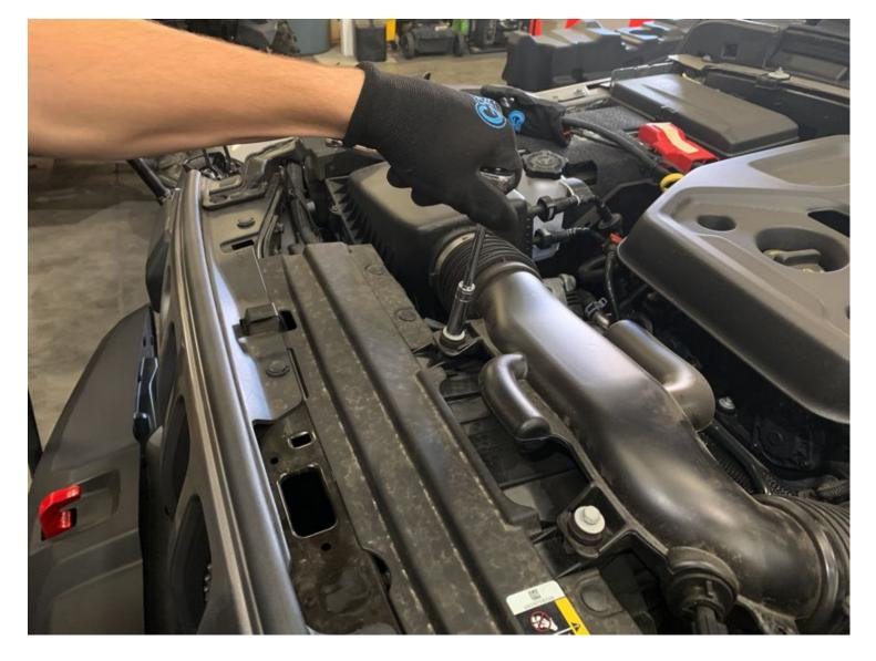
Remove the two bolts securing the stock intake tube to the fan shroud.
