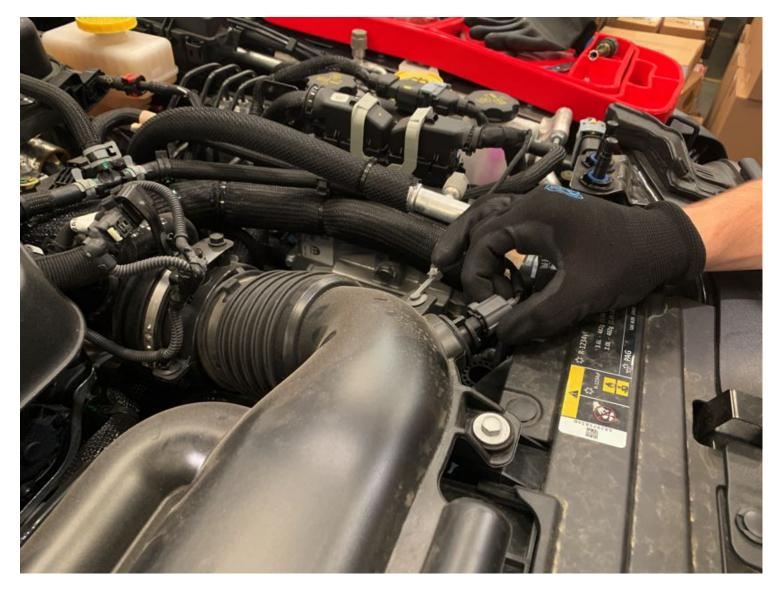
Disconnect the IAT electrical harness from the IAT sensor by pressing down on the locking tab and pulling off the IAT sensor connector.
