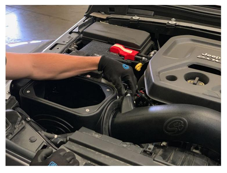
Reconnect the CCV and Vacuum fittings onto the 1/2" and 3/8" Quick Connect Fittings (H & I). You should hear a click when the CCV and Vacuum fittings are fully secured.
