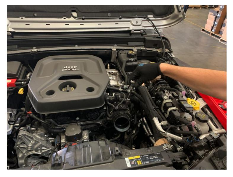
Remove the two bolts securing the wire harness bracket to the turbo resonator chamber.
