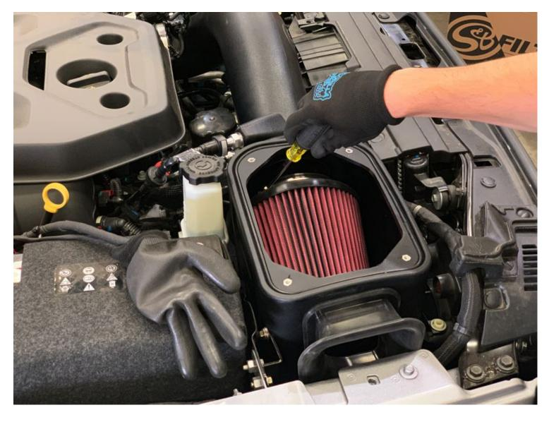
Install the Air Filter (E) and #80 Hose Clamp (M) onto the Intake Tube (B) then tighten the hose clamp. Do not overtighten.
