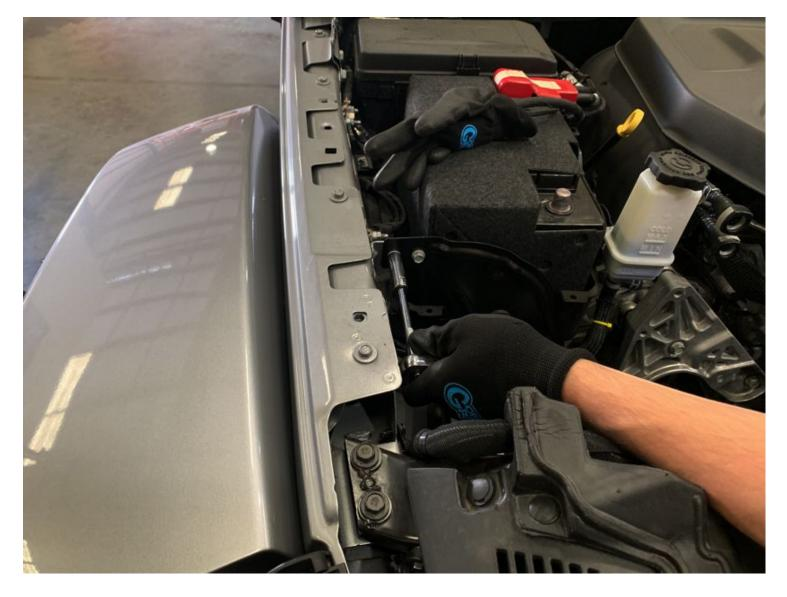
Remove the bolt, closest to the fender, from the battery tray bracket.
