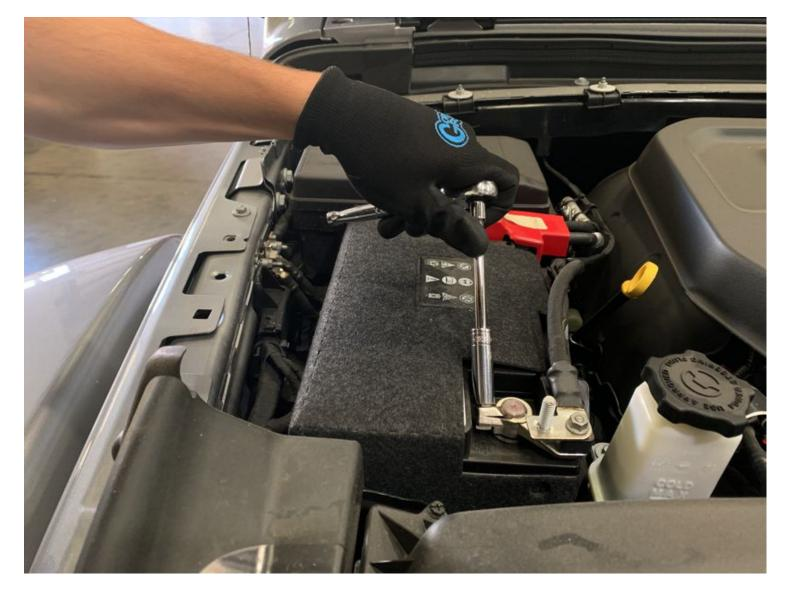
With the ignition switched off and the parking brake set. Disconnect the negative battery cable on the passenger side. **Note:** Failure to disconnect the battery may cause the CEL to illuminate upon completion of the installation and subsequent operation. Do not skip this step!
