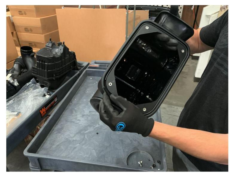
Install the Lid Seal (F) into the groove on top of the Intake Box (A). Cut away any excess lid seal.
