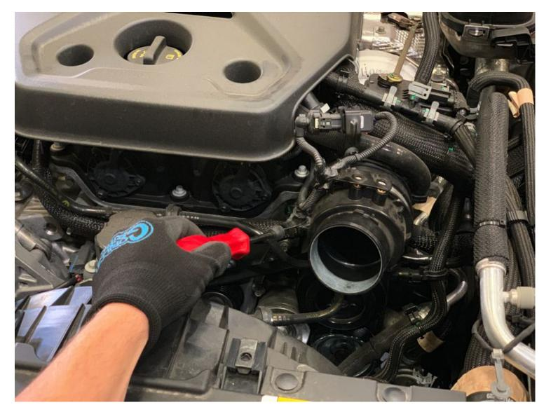
Disconnect the clip securing the wire harness to the turbo resonator.
