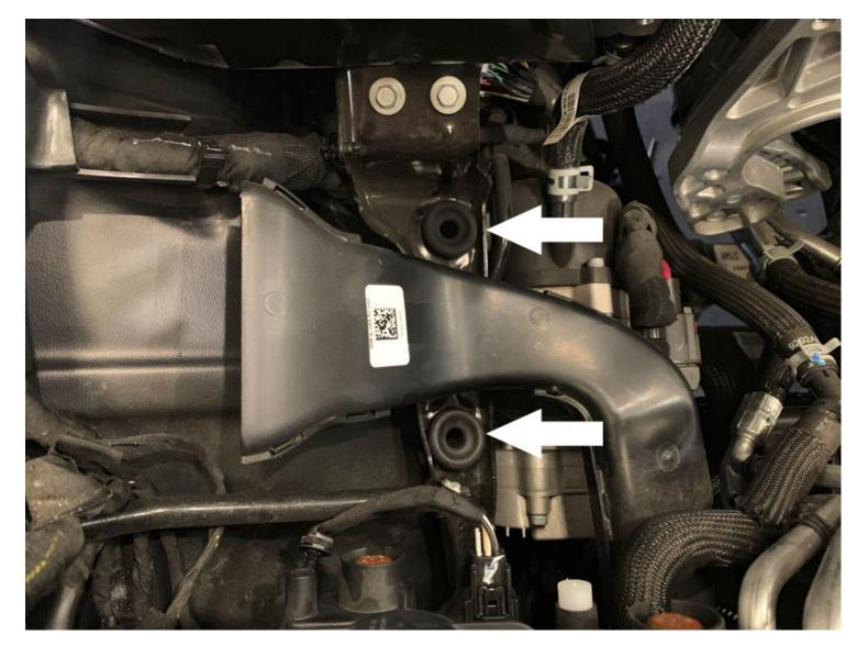
Check to make sure the two grommets are still in place in the vehicle. If they are missing, they were probably removed with the stock intake box. If the grommets came out of the vehicle with the stock intake box, remove the grommets from the stock intake box and reinstall into the vehicle.
