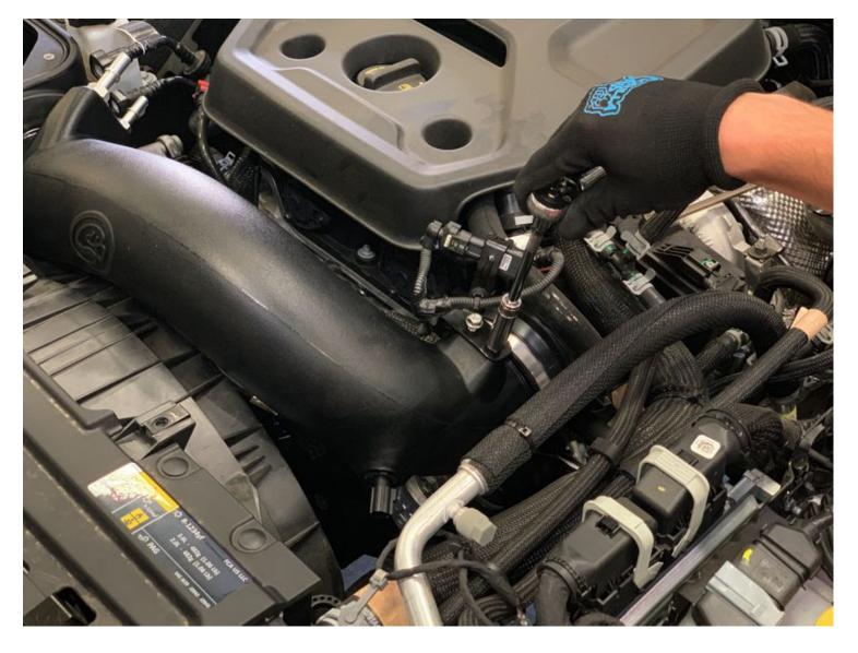
Install the wire harness bracket onto the Intake Tube (B) with the M6 Bolts (L).
