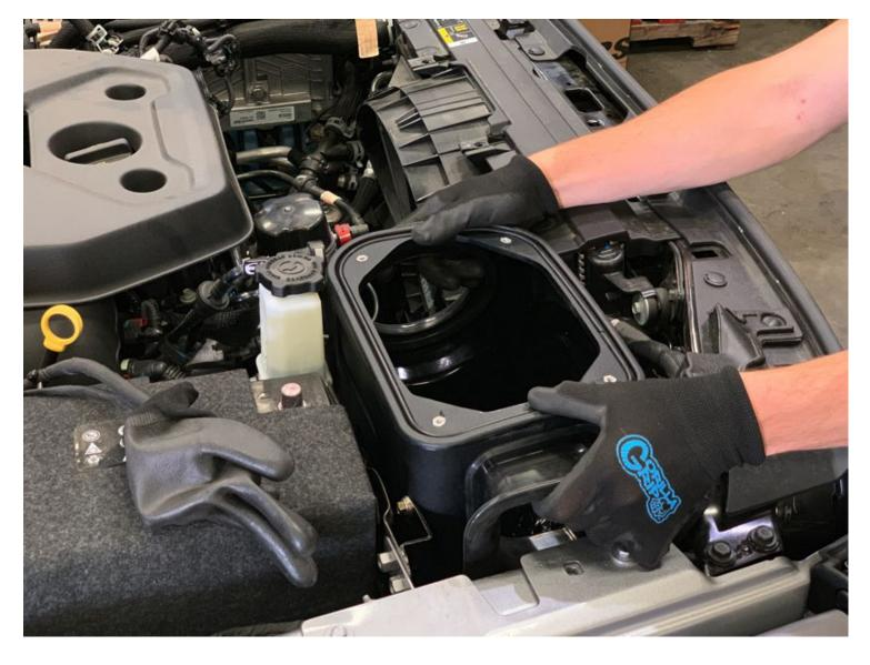
Install the Intake Box (A) into the vehicle, making sure the prongs align with the two grommets, then push down on the intake box to fully seat the prongs.
