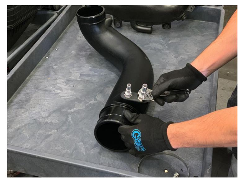
Install both the 1/2" and 3/8" Quick Connect Fittings (H & I) into the Intake Tube (B) until finger tight then, with a crescent wrench, tighten the fitting an additional one to two complete turns.
