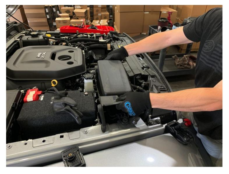
Lift the stock intake box to unseat the prongs from the grommets then remove the stock intake box from the vehicle.
