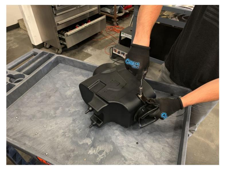
Install and tighten the Bracket (K) with the M6 Bolt (L) and M6 Washer (Q) onto the Intake Box (A). Do not overtighten.
