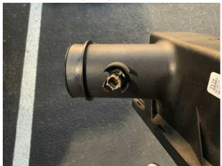
Install the IAT Sensor Grommet (T) into the IAT sensor adapter plate (Q).
