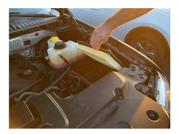
Remove 10mm nut holding down the hood sensor bracket, and move the bracket aside. This will allow access to the 13mm bolt on the factory airbox. Tools Required: 10mm wrench or socket
