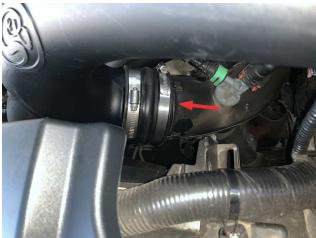
Insert the top turbo inlet tube completely and tighten the #56 hose clamp (F). Tools Required: 5/16" nut driver or similar tool.
