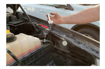
Attach coupler (P) to intake tube (K) using 2 #56 hose clamps (F). Only tighten the hose clamp on the S&B intake tube side while leaving the other hose clamp loose. Tools Required: 5/16" nut driver or similar tool.
