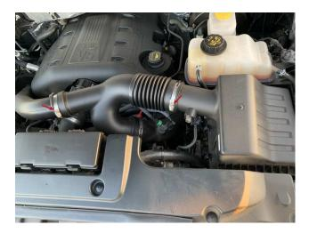
Pull back on the bellowed portion of the intake tube, removing it from the stock airbox cover.
