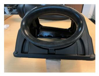
Insert the intake tube (K) into the cuff. Ensure that the tube is pushed all the way to the stop hump of the tube. This will not be an air tight fit to allow for engine movement.
