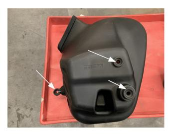
Remove the top portion of the factory scoop by prying the tabs to the sides of the scoop from the factory intake assembly using a flathead screwdriver.
