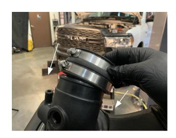
Attach the mounting bracket (G) to S&B airbox (K) by securing the  $\frac{1}{4}$ "-20 screws (D) and  $\frac{1}{4}$ " washers (E) first by hand tightening
