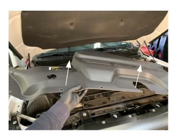
Remove the 2 bolts attaching the factory air scoop to the vehicle using a 10mm socket and driver. Collect these bolts and set them to the side, to be re-installed later.
