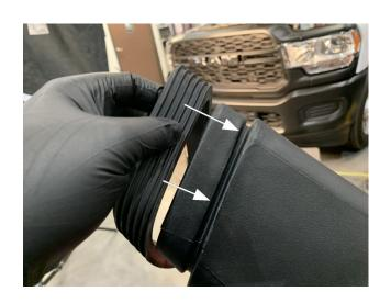
Assemble the Silicone tube seal (L) onto the S&B Airbox (K)
