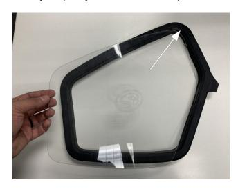
Install the S&B Snap-in Clear Lid onto the S&B Airbox by inserting one corner or edge of the seal fully first, then work around the lid pressing on each side.
