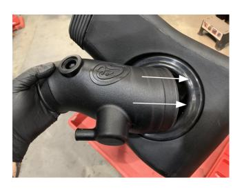
**STEP 14**Assemble the IAT Grommet (N) onto the S&B Tube (M)
