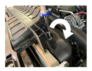
Drop the Silicone S&B Air Filter (C) into the S&B Airbox (K) with the #88 hose clamp (J) attached loosely. Enter the airbox by the filter flange first, this will make it easier to align the filter flange onto the tube. Slide the lower inner filter flange lip under the tube and push in firmly over the tube.
