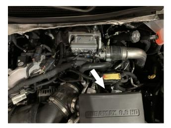
Loosen the hose clamps connecting the intake tube to the airbox and plastic turbo adapter. Then remove the intake tube from the vehicle. **Tools Required:** Socket Wrench, 8mm Socket.
