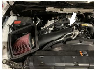
Verify that the tube seal completely seals around the complete circumference of the intake tube and then tighten the two #54 hose clamps found around the coupler. **Tools Required:** Socket Wrench, 5/16" Socket
