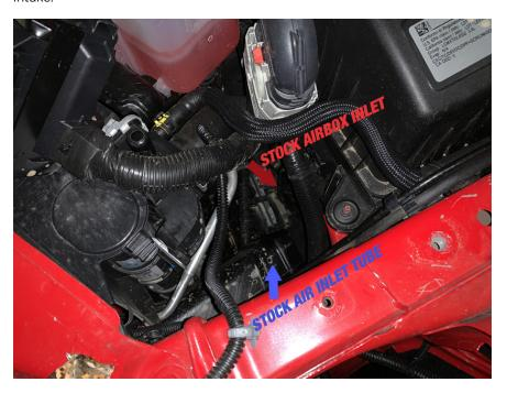
Carefully disconnect the large wire harness at the front of the air intake. The snap feature is designed to release under sufficient upward force, however, pulling upward while tilting the harness toward the rear of the vehicle will help disconnect the harness.
