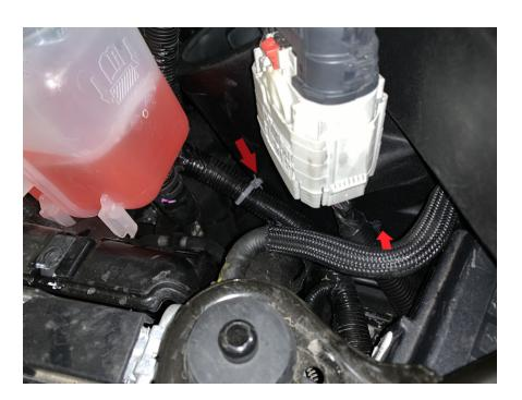
Reinstall the bolt holding down the front coolant reservoir. Tool Needed 10mm socket or wrench.
