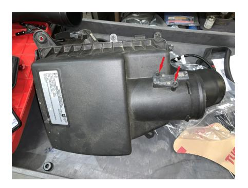
Find the Short S&B Intake Tube (2) and HP1407-00. Install the MAF Sensor into the Short S&B Intake Tube using the MAF Pad (9), MAF Gasket (10), and supplied screws (11). Take care that the MAF pad and sensor are oriented correctly on the MAF boss on the tube, as shown.Tool Needed: Philips Head Screwdriver
