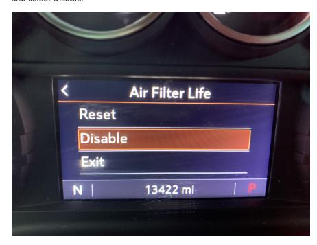
The screen should now display "Disabled", as shown. Please verify the screen still shows disabled after the battery disconnect has been completed. If not, please repeat the process.
