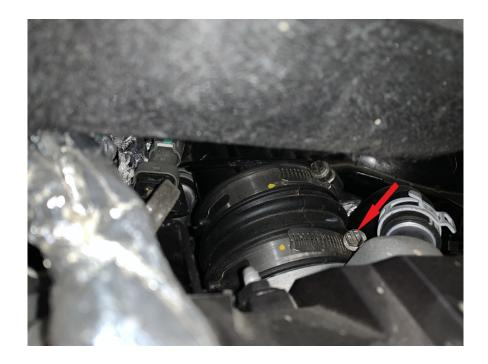
Lift upward on the intake tube, until you feel it release. There is a mounting point with a grommet molded into the intake tube, this must be dislodged before the tube can be removed. Once the tube is free, the easiest way to remove it is by pulling it toward the driver's side and pulling it through the area where the coolant reservoir was.
