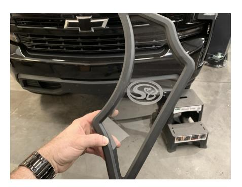
Install the lid and lid seal into the airbox starting from the tight corners and curved edge, working to the straight side.
