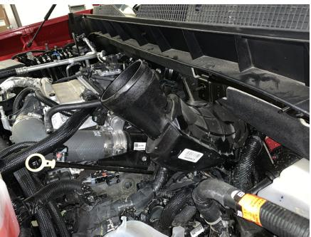
Find the long S&B Intake tube (3) and the mounting bracket hardware kit (HP1725-00). Attach the small grommet (26) to the bracket (27) and the bracket to the tube with the  $\frac{1}{4}$  x 20 Button Head Cap Screws (17).Tool Needed:  $\frac{5}{32}$ " or 4mm Hex Key.
