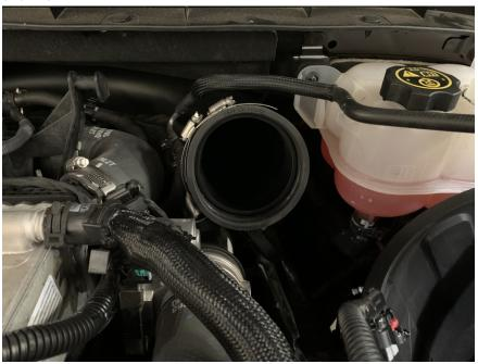
Find the S&B Air Filter (2) and snap the filter into the airbox. The installation is easiest when the snap is chased around the perimeter of the filter base, starting with the lowest point of the filter. Attach the #88 Hose Clamp (22) if not already attached.
