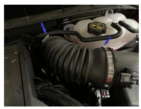
Loosen the nut with a captive washer holding down the stock air box. Set aside the nut for reuse. Tool Needed: 10mm wrench or socket.
