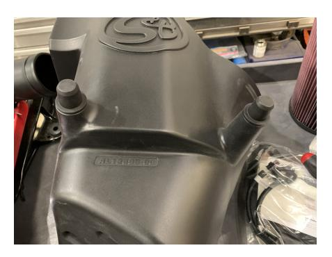
Install the Airbox into the vehicle, sliding the prongs into their holes and lowering Separate the box onto the stud. Loosely Reinstall the nut with a captive washer onto the stud. two apart.
