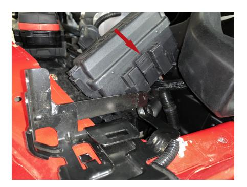
Reinstall the fuse box bracket. Ensure the fuse box is near, but not attached to the bracket. Tool Needed: 10mm wrench.
