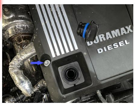
Remove the bolt holding down the rear coolant reservoir. Let the reservoir rest where the stock air box was formerly located. If you wish to disconnect either of the this hose clamp is very limited, caution and patience are required. Tool Needed: overflow lines, be sure to unscrew the cap to relieve the pressure in the reservoir.
