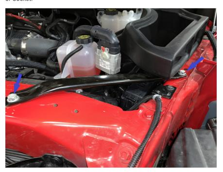
stock air inlet tube should be touching the seal when fully inserted. It may be helpful Tool Needed: 13mm Wrench or Socket. to guide the tube with one hand inside the air box.
