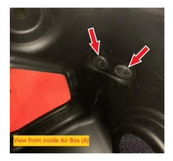
From the inside of the Air Box (A), install Shoulder Bushings (F) into the Grommets (E)
