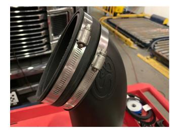
Insert the Intake Tube (T) into the Box Seal (M) located on the Air Box (A). Work the Intake Tube (T) slowly, at the angle shown, until the bead on the Tube is up against the Box Seal (M).
