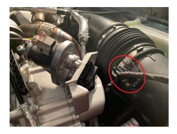
Remove the ribbed push in clip on the wiring harness from the stock intake lid.
