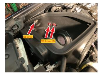
Tighten the screw that was hand tightened in Step 21 to secure the Air Box Bracket (H) to the fender frame.
