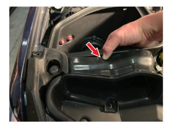
Secure the Air Box Inlet (P) onto the vehicle with the push in rivet removed in Step 8. Make sure the push in rivet is fully inserted and the center stem pushed all the way down.
