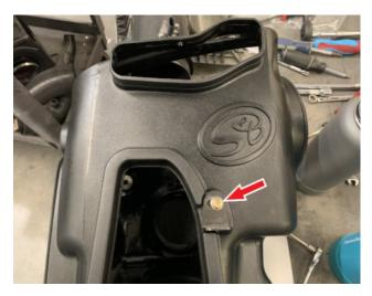
Install Washer (D) to the bottom of Air Box (A) using Hex Flange Bolt (C).
