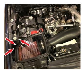
Inspect your installation, make sure the kit is properly positioned and all fasteners and hose clamps are secured. Keep all stock parts in case you would ever need to reinstall the stock intake assembly. Affix the ID label near the Intake kit. If you are an installer, give the owner the QR code for the Installation Instructions so that he/she is aware of the Maintenance and Operation procedures given at the beginning of the Instructions. The installation is now complete.
