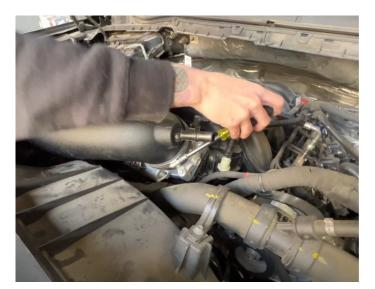
Tighten the clamp at the filter.
