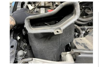
Remove the stock front inlet and box out from the vehicle.
