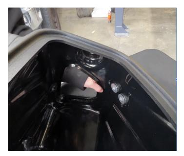
From the inside of the Air Box install Shoulder Bushings into the Grommets.
