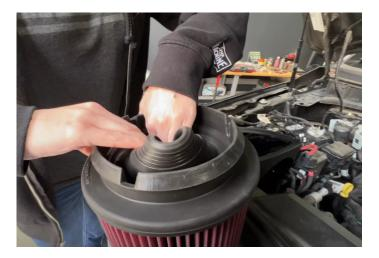
Insert the Filter with Hose Clamp into the Air Box with the Filter flange pointing up.
