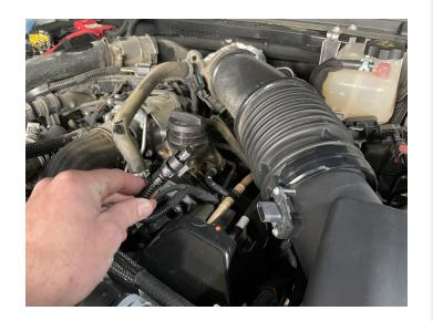
Remove the bolt that secures the factory air box to the fender of the jeep. This bolt will be reused with the new S&B kit.
