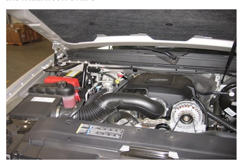
With the ignition switched off and the parking brake set, disconnect the negative battery cable on the battery.
