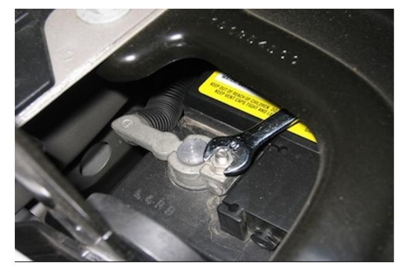
After the batteries have been disconnected for at least 2 hours, reconnect the positive battery terminal on the passenger side first then reconnect the negative terminals.
