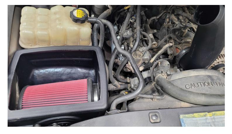
Work the Air Box (E) into the Vehicle. Align the four holes with the OE Mounting location and secure using OE bolts or supplied Allen head screws (H) and ss washers(G). Place S&B Filter (c) inside of Air Box (E).
