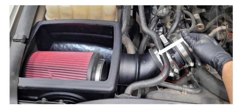
Connect the MAF sensor Assembly (Step 15) to the Filter to MAF Tube (J or Q) and secure using a #50 Hose Clamp (K).
