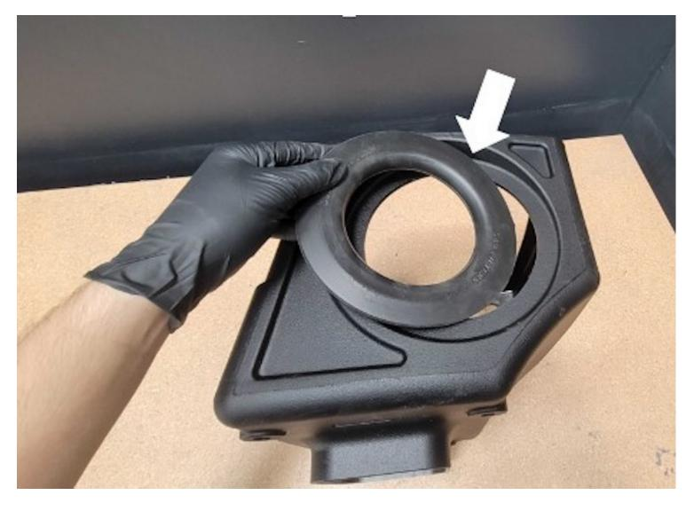
Install Box Seal (I) to the S&B intake Air Box (E). Make sure that the Air Box (E) is fully seated into the groove of Box Seal (I).
