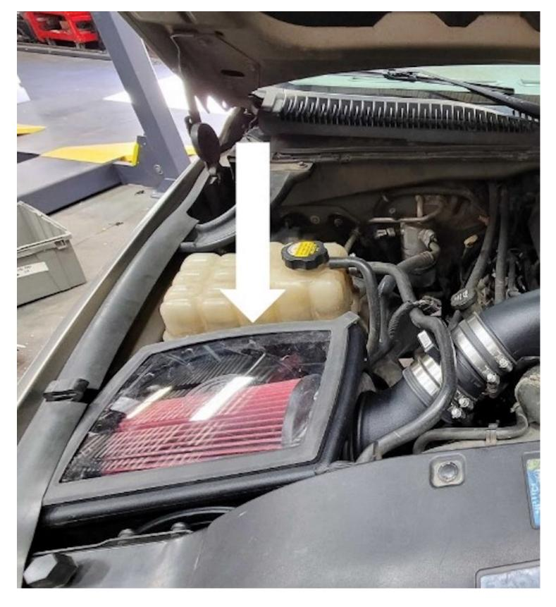
Install the polycarbonate Lid (A) with Snap-In Lid Seal (B) onto the Intake Box (E). start by inserting the Lid seal groove over the Air box opening on one corner first and then work your way around the Air Box. Make sure that the Lid seal groove snaps over the entire Air Box opening. Check all around the Lid seal snap groove to make sure it has snapped over the entire Air Box opening.
