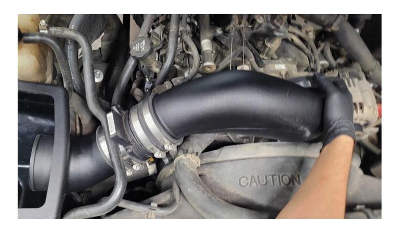
Position the Silicon Coupler (N) end of the over the throttle body and firmly secure the #72 Hose Clamp (D), then secure the #50 Hose Clamp (K) at the Straight Coupler.
