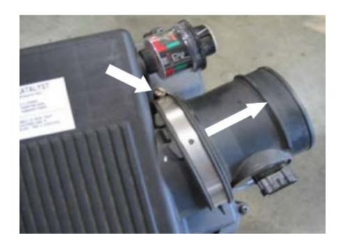
Loosen the hose clamp on the OE airbox and remove the MAF sensor. Note the direction of the airflow through the sensor.
