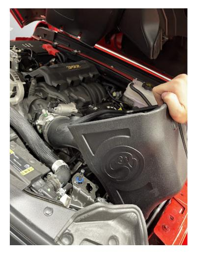
First, make sure all 3 rubber grommets did not get pulled off from removing the stock airbox previously. Slide S&B coupler onto throttle body first at a downward angle, then push airbox straight down into stock rubber grommets.
