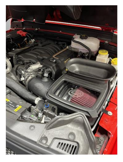
Inspect your installation. Make sure the kit is properly positioned and all fasteners and hose clamps are secured. Keep all stock parts in the event you would ever need to reinstall the stock intake assembly. If you are an installer, give the owner the QR code for the Installation Instructions so that he/she is aware of the Maintenance and Operation procedures. The installation is now complete.
