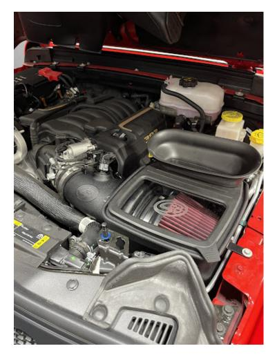
Tighten both clamps on the throttle body and S&B tube using a 5/16" wrench or flat head screwdriver.
