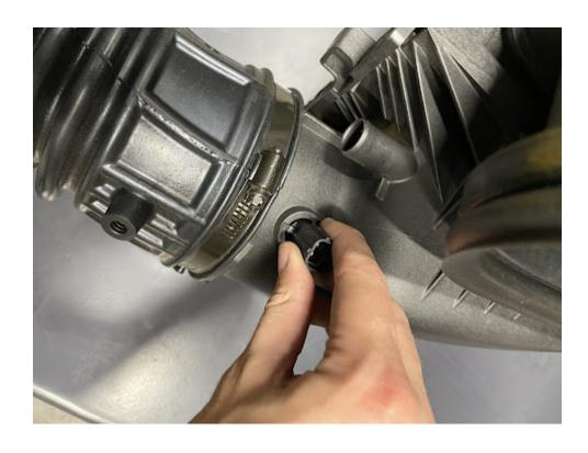
Transfer the IAT sensor from the OEM tube into the S&B tube as shown. The locking tab should rotate over the ramp and lock into position, use the turn arrow for indication.
