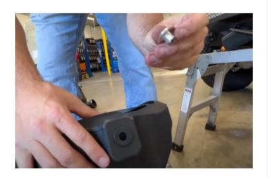
Install the scoop onto the S&B airbox using the provided push rivets.
