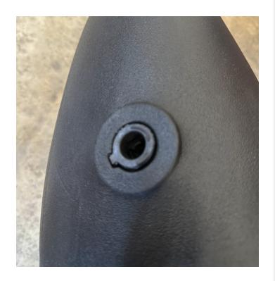
Thread the small insert into the S&B intake tube. The insert is NPT so there will be some thread showing.
