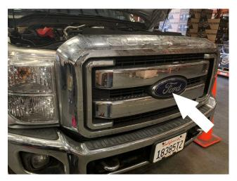
Finish reinstallation of the grill by replacing the four screws removed in step 9.
