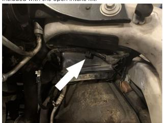
Install the provided grommet (E) into the hole on the intake tube support bracket (D) and attach it to the frame of the vehicle in the position shown. Using one of the screws that was removed in step 7, loosely tighten the bracket down so that there remains some play.
