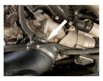
Visually inspect the installation of the intake kit. Make sure the tube is fully seated within the support tube and that the tube did not push out the grommet during installation. The picture provided shows a good place to inspect the tube's installation.
