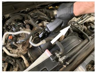
Remove the two screws securing the bracket under the airbox which holds the grommets to seat the airbox. Then remove the bracket from the vehicle. We will reuse one of the removed screws in step 10. Tools Required: Socket Wrench, ½" Socket
