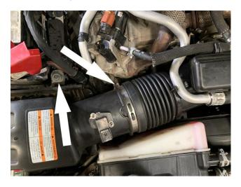
Loosen the hose clamp at the turbo inlet and remove the screw securing the stock intake tube. Tools Required: Socket Wrench, 8mm Socket
