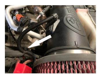
Wrap the metal coolant line that sits on top of the tube with the provided foam wrap (L) to protect your intake tube from being scratched or rubbed by the metal coolant line.
