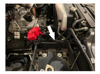
Pop out the two harness clips on the back of the battery tray.
