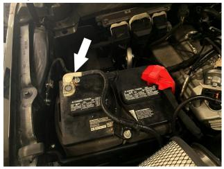
Zip tie the slack of the MAF cable to the indicated places to make sure it does not move during operation of the vehicle.
