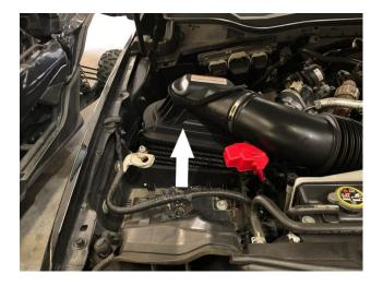
Disengage the red locking clip, press down on the tab, then pull out to disconnect the MAF sensor harness from The MAF sensor.
