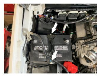
We will now rearrange and flip the tightening mechanism on the negative battery cable terminal. This will allow the terminal to reach the battery post after the battery relocation. First completely remove the nut, screw and wedge then pull out the metal clip then reinstall the metal clip into the longer side on the battery terminal as shown.
