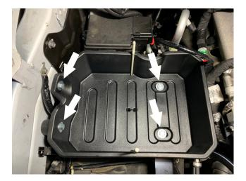
Fully tighten the center mounting hole with the M8 Screw (M), Washers (O) and M8 Locknut (L) on the Battery Tray Bracket (K) then remove the two stock screws from the bracket.
