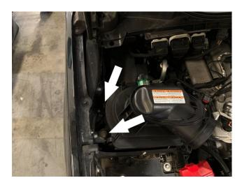
Pop out the harness clip attached to the back of the stock intake box.
