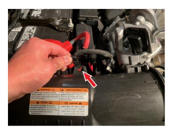
Loosen the hose clamps on the intake tube connected to the turbo inlet and intake box.
