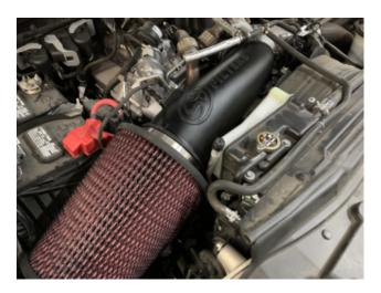
Finish securing the kit to the vehicle by tightening the #74 hose clamp over the coupler and around the turbo inlet.
