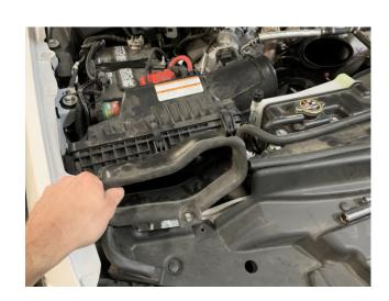
Using socket extension(s), remove the screw holding the stock intake box to the grill inlet duct.
