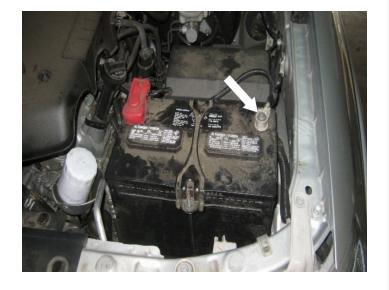
Remove the two nuts securing engine cover then lift up and remove the engine cover from the vehicle. Set one of the nuts aside, the hardware will be reused in Step 18.
