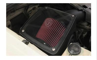
Inspect your installation, make sure the kit is properly positioned and all fasteners are secured. Keep all stock parts in case you would ever need to reinstall the stock intake assembly. Affix the ID label near the intake kit. The installation is now complete.
