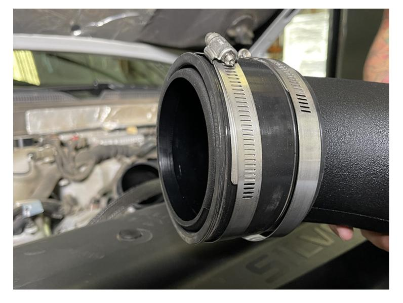
Install the Coupler (H) with #64 Hose Clamps (G) onto the Intake Tube (C). Slide the coupler as far up the intake tube as possible. Do not tighten the hose clamps at this time.
