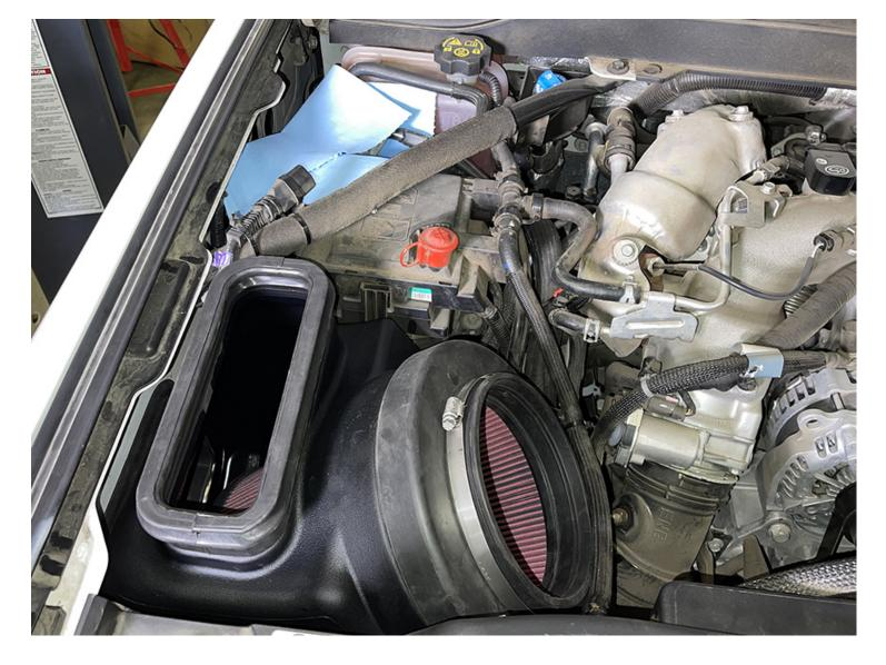
Install the filter (B) into the intake box (A). The lip of the filter should go over the flange on the box and snap onto it.
