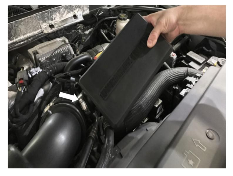
Loosen the hose clamp at the resonator then remove the resonator from the intake tube.
