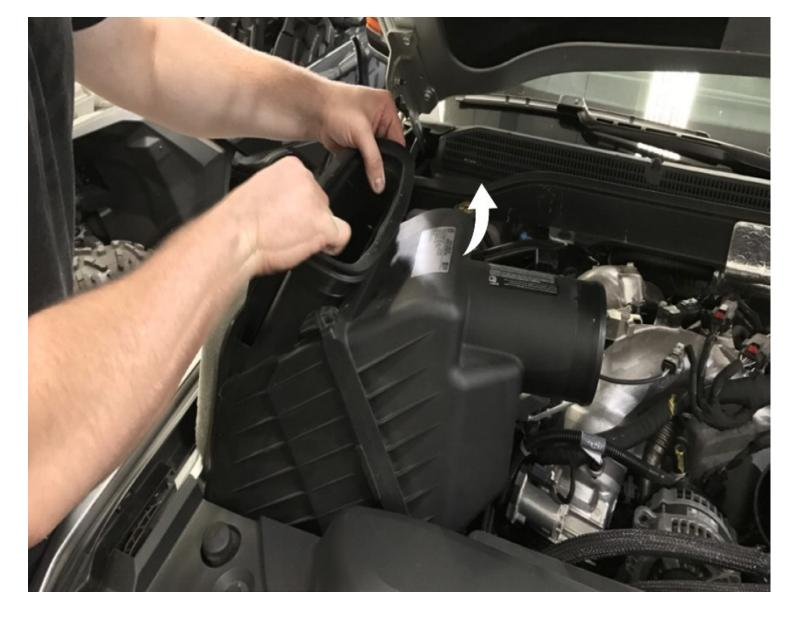
Lift the intake box to pull the prongs from the grommets and remove the intake box from the vehicle.
