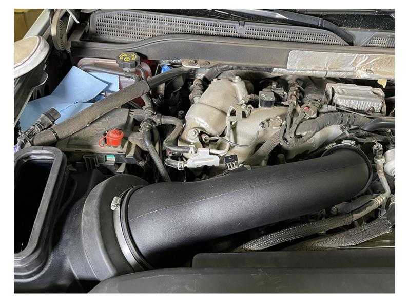
Insert the intake tube (C) into the filter (B). Align the turbo side with the turbo inlet and slide the coupler (H) down over the turbo inlet. Tighten the hose clamps at the filter and turbo sides of the tube.
