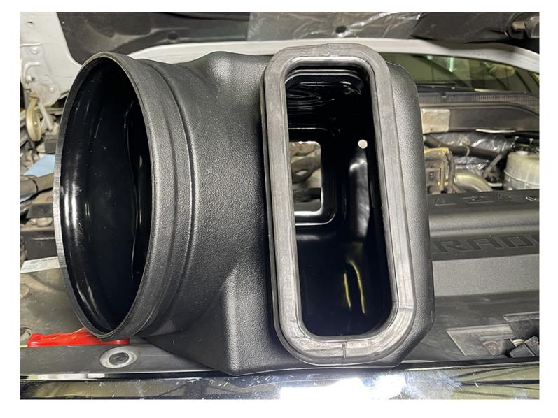
Install the scoop seal (J) onto the intake box(A).
