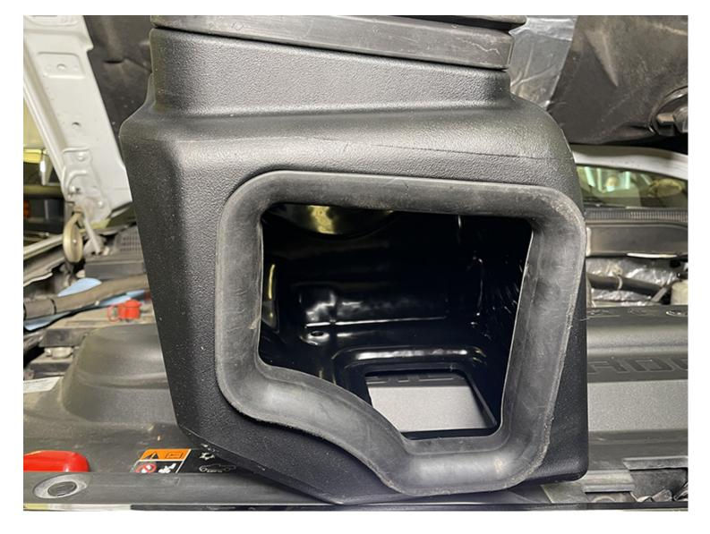
Install the Fender Seal (K) onto the Intake Box(A).
