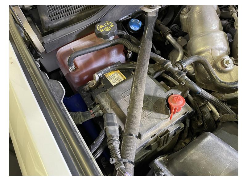
Reconnect the negative battery terminals on both batteries. Inspect your installation, make sure the kit is properly positioned and all fasteners are secure. Keep all stock parts in case you ever need to reinstall the stock intake assembly. Affix the ID label near the intake kit. The installation is now complete.
