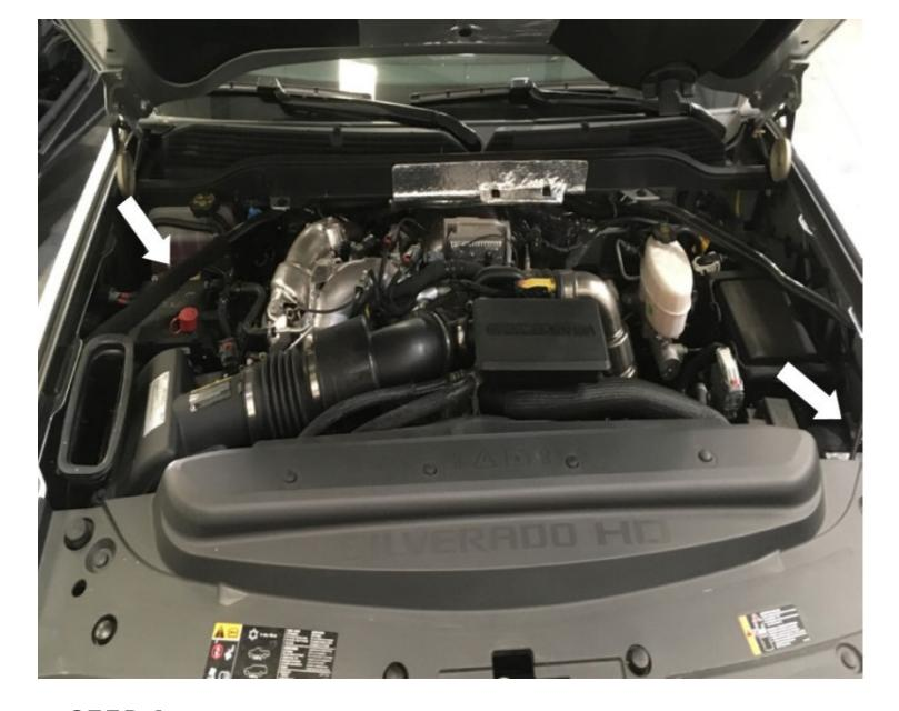
With the ignition switched off and the parking brake set, disconnect the negative battery cables on both batteries.
