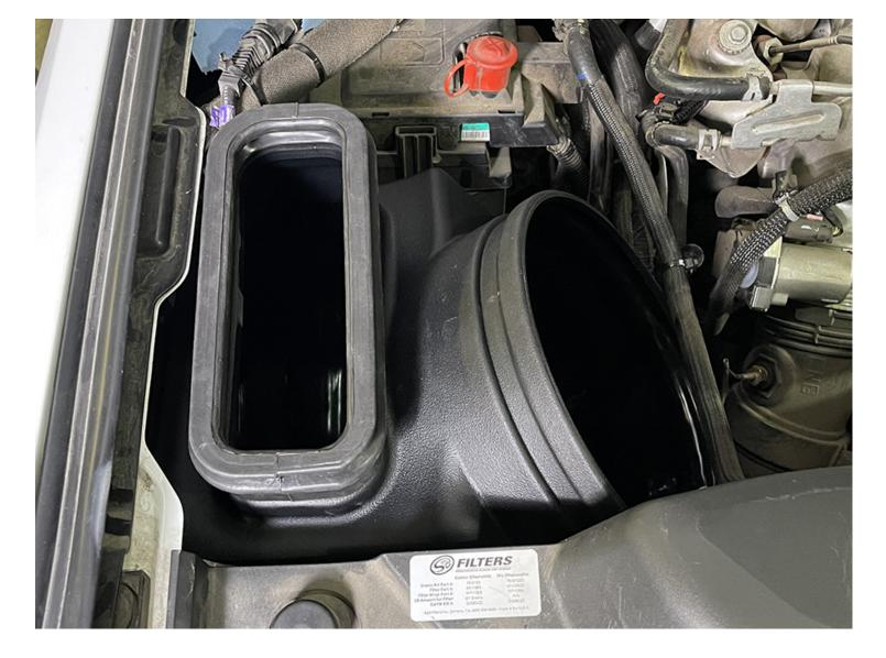
Place the Intake Box (A) into the vehicle.
