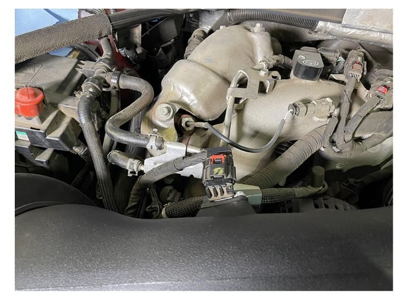
Reconnect the electrical harness into the MAF sensor and engage the red locking clip.
