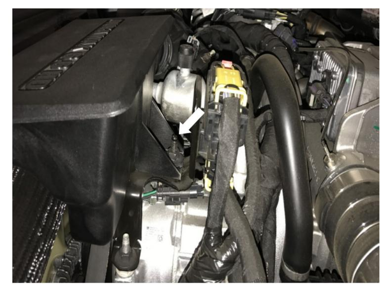
Remove the nut securing the stock resonator.
