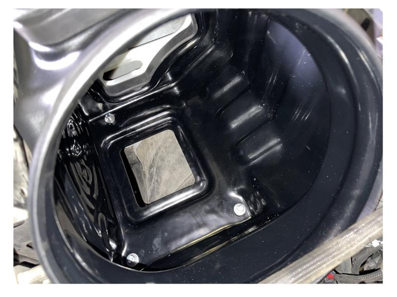
Align the holes on the Intake Box with the mounting holes on the vehicle then install the three M6 Bolts (N) and Washers (M) and tighten.
