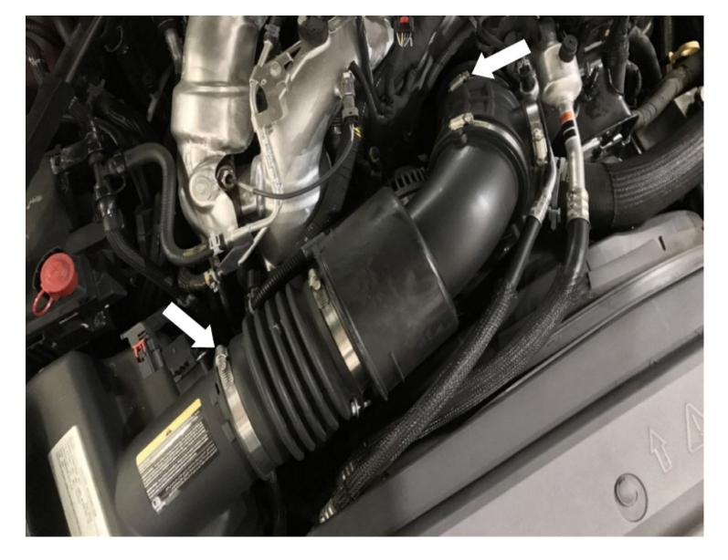
Loosen the hose clamp at the turbo inlet and intake box then remove the intake tube from the vehicle.
