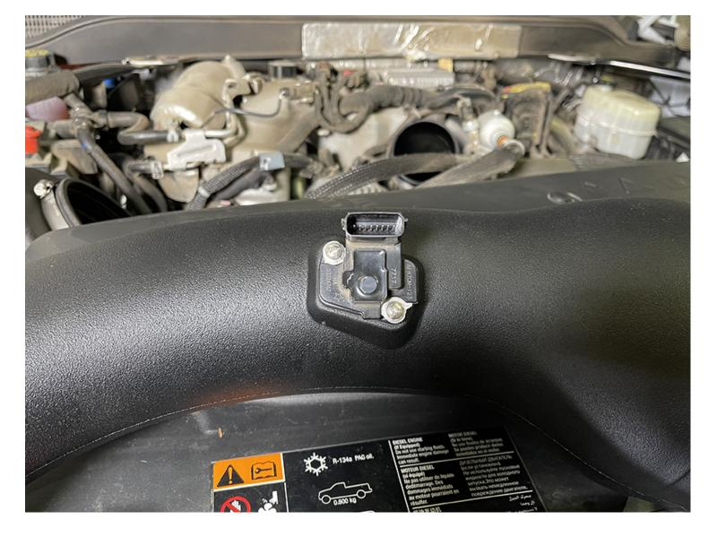
Carefully remove the MAF sensor from the stock intake tube then install the sensor onto the S&B Intake Tube (C) with the #8-32 Screws (F), MAF Plate (E) and MAF Gasket (D).
