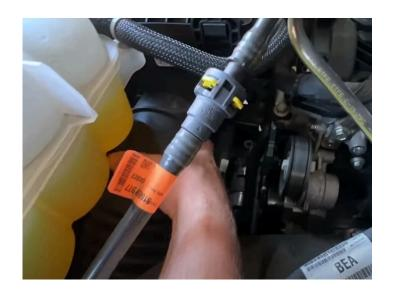
Remove the IAT sensor from the airbox. Lift the tab up over the ramp and rotate counterclockwise
