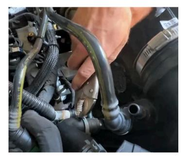
Use a 5/8" quick disconnect tool to remove the line on the tube.
