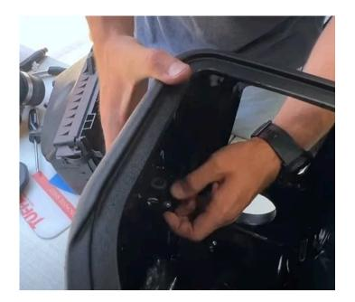
Install the tube seal into the S&B Air Box.
