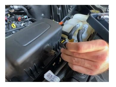
With a 10mm socket, remove the nut holding down the airbox.
