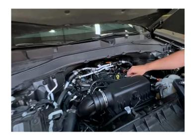
Remove the white PCV connector by depressing the button and pulling off
