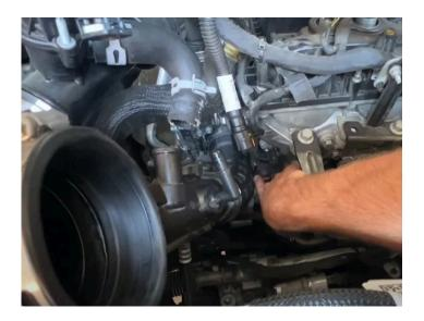
After the complete OEM intake system is removed, we will be assembling the S&B intake. Start by installing the antilag coupler into the intake tube. Install the straight coupler onto the intake tube.
