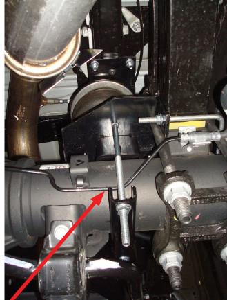
If the hard brake line is resting on the lower bracket carriage bolts on either side, push or pull the brake line out of the way.
