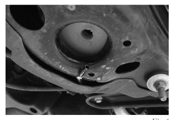
7. Install the air line onto the air spring (Fig. 7) and ensure the clamp is in the proper position using needle nose pliers (Fig. 8).
