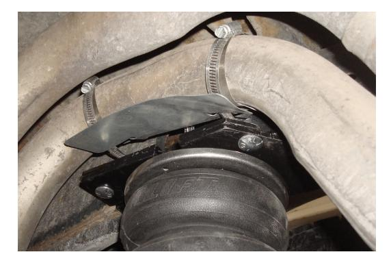
2. Bend the heat shield up so that it is between the pipe and the air line (as shown in the photo).
