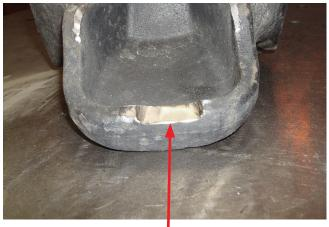
Grind out area between marks made from ABS bracket as shown.
