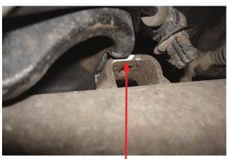
Grind strike plate so that there is clearance between Fig. 7 the ABS bracket and strike plate when spacer is sitting on the spring perch.
