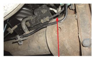
Look for rubbing from modification made to brake components. Adjust where necessary.
