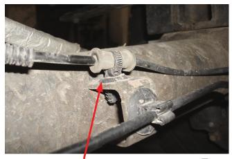
Pull the tree mount holding the ABS line, out of the  $\it Fig.~10$  top mounting of the bracket.
