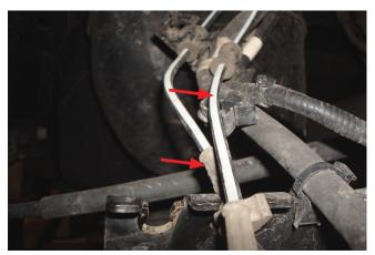
Pull the ABS lines out and away from the left side of the bracket bolted to the axle.
