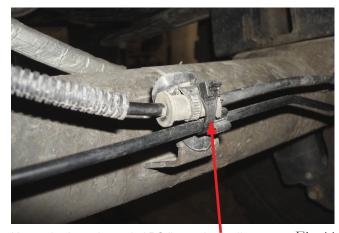
Use a zip tie and attach ABS line to brake line as shown.
