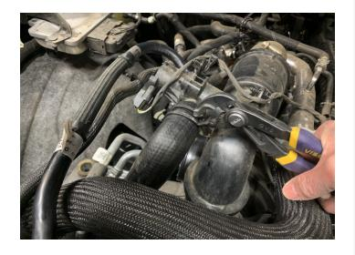
Remove the larger vapor quick connect fitting from the intake tube. Pull out the green locking tab then depress the white release clip and remove the quick connect fitting.
