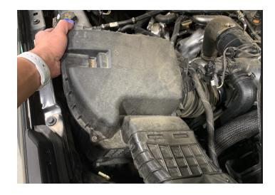
Make sure the bottom box grommets stayed in the vehicle and did not get pulled out with the intake box.
