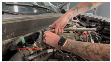
Now that you have removed the (2) nuts, you may successfully disconnect the electrical sensor and remove the retainer clips.
