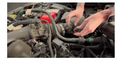
Now that the intake tube hose-clamp has been loosened, you may successfully remove the Airbox from the vehicle
