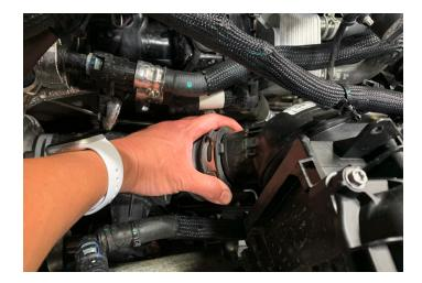
Remove the screw that mounts the rear corner of the intake box to the fender frame. Set the screw aside to be used later.
