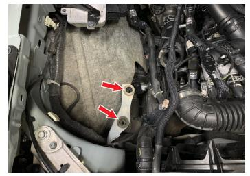
Loosen and remove the (4) screws holding down the charge air pipe. Set the screws aside to be reused later.
