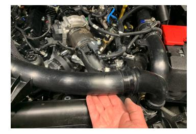
Squeeze the by-pass hose quick connect collar to release the locking tabs and remove the hose from the long intake tube. Set the by-pass hose aside.
