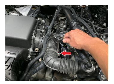
Remove hose from the intake box and position it aside.
